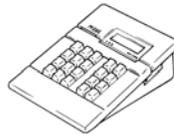
**Mini Mars-2 Controller** — for automatic reading of 16 mm Cartridge Microfilm using up to 2-level image marks.
